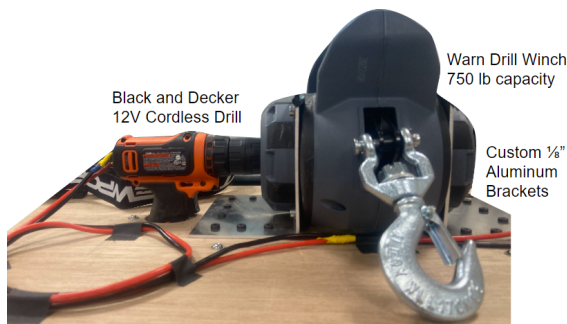
Fig. 8. Winch assembly, driven by cordless drill and attached to the marine plywood deck of the boat with custom brackets.
