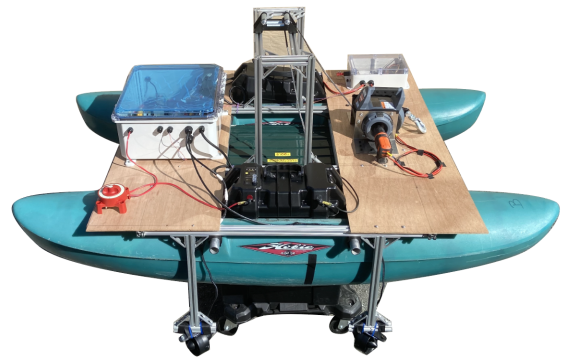
Fig. 9. Completed platform, including electronics boxes, batteries, winch, and sampling frame.
