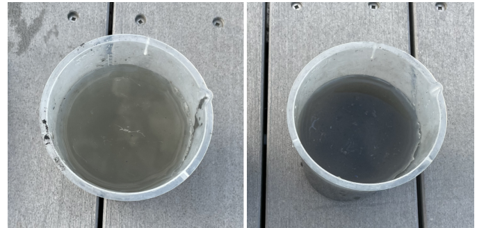
Fig. 12. Water collected using the core catcher and ball valve (left) and water collected using the same core catcher and flap valve (right).
